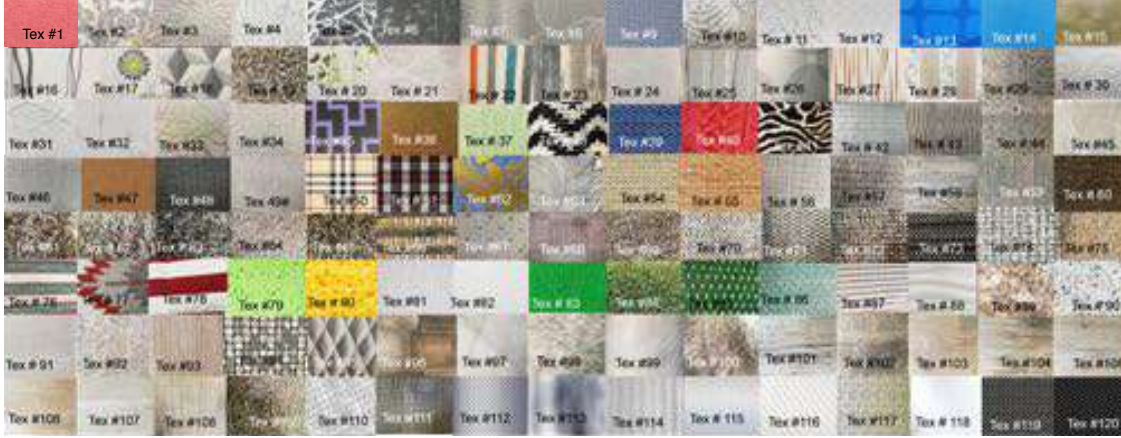
FIGURE 3.3. The selected experimental materials consist of 120 different natural and synthetic textures with uniform (regular) and non-uniform (irregular) structures including: Papers and vinyl wallpapers (Tex.#1-Tex.#37), Textiles (Tex.#38-Tex.#57), Carpets and mats (Tex.#58-Tex.#78), Foams and sponges (Tex.#79-Tex.#82), Fibers (Tex.#83, Tex.#84), PVC and rubber type surfaces (Tex.#85-Tex.#95), Leathers and furs (Tex.#96-Tex.#100), Wooden surfaces (Tex.#101-Tex.#109), metal surfaces (Tex.#110-Tex.#113), Fibreglass and glass surfaces (Tex.#114-Tex.#118), and Carbon sheets (Tex.#119, Tex.#120). All materials acquired from Bauhaus ( www.bauhaus.info ).
