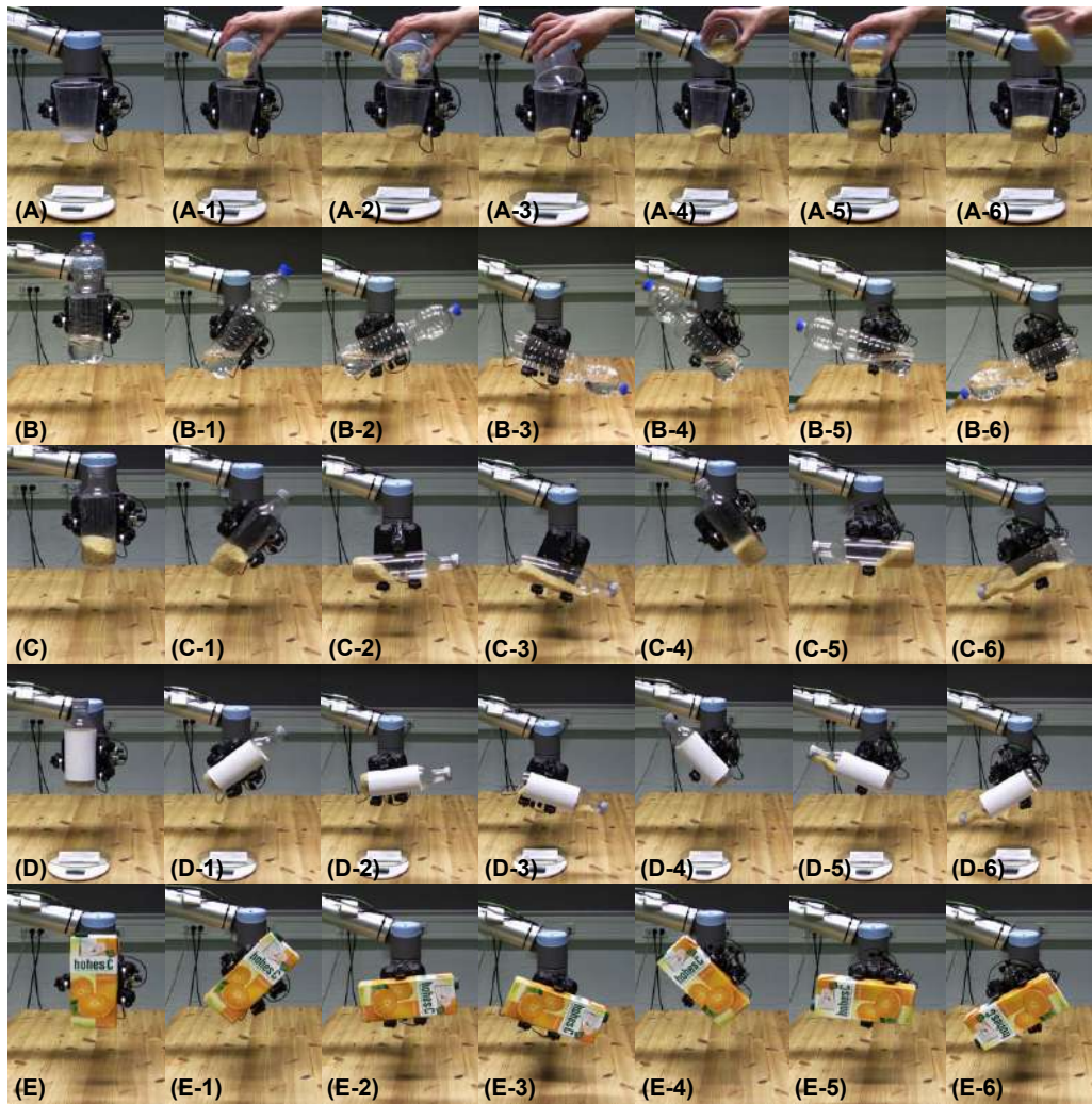
FIGURE 8.8. Manipulation of deformable objects with different characteristics, such as stiffness, surface texture, and center of mass, using Algorithm 8.1.
