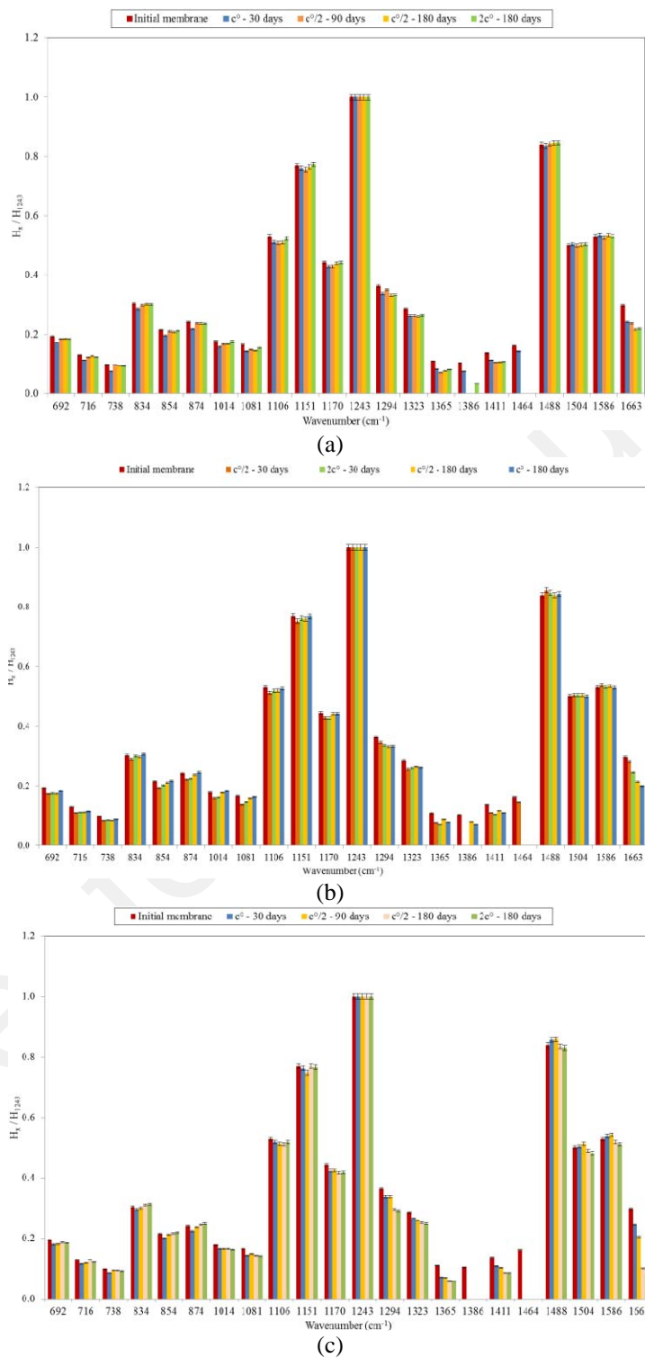
Fig. 1 Ratios H_x / H_{1243} used for the identification of the chemical bonds the most affected by P3-Ultrasil 110 ageing (a), by P3-Ultrasil 75 ageing (b), and P3-Ultrasil 67/69N ageing (c)
