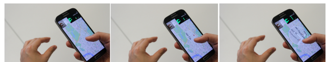
Figure 14: The size of magnifier on the map can be adjusted continuously by the transitions between PinchOpen and PinchClose gesture pair.
