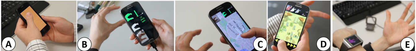
Figure 1: Touch input is expressive but can occlude large parts of the screen (A). We propose a machine learning based algorithm for gesture recognition expanding the interaction space around the mobile device (B), adding in-air gestures and hand-part tracking (D) to commodity off-the-shelf mobile devices, relying only on the device's camera (and no hardware modifications). We demonstrate a number of compelling interactive scenarios including bi-manual input to mapping and gaming applications (C+D). The algorithm runs in real time and can even be used on ultra-mobile devices such as smartwatches (E).
