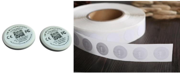
Figure 4.2. Examples of readily available commercial BLE disk beacons and NFC sticker tags.
