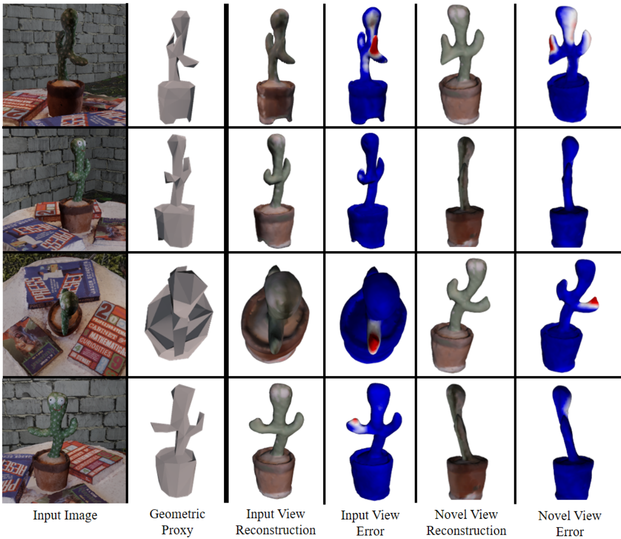
Figure 5.5: Results for our Cactus sequence. We include error coloring where blue is zero error and red is high error, relative to the entire sequence.
