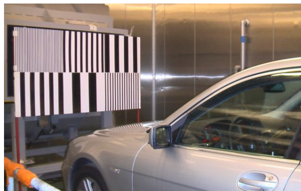
Figure 1. The configuration of our experiment, a car and a background board in a wind tunnel room.
