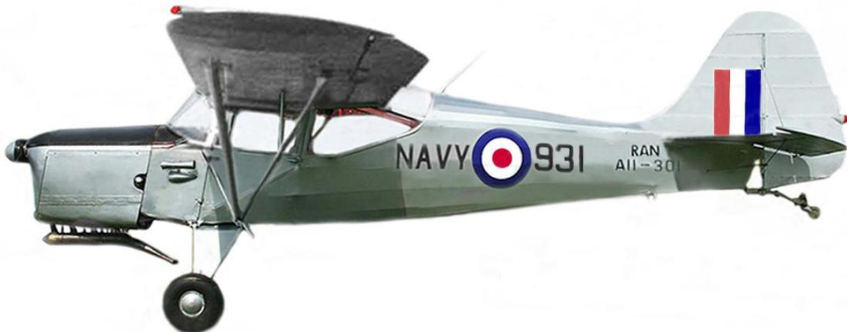
**A11-301 (c/n 3064):** was coded 931 (above) then 857 (below) in 9" x 6" figures, and sold in OCT 1963 as VH-MRD, but was fitted with a horizontally opposed engine that changes the appearance and remains airworthy.
