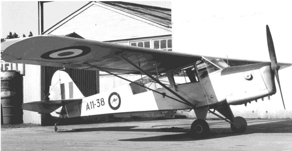
**'Type-D' and kangaroo roundel sizes: diameter inches (cm): fuselage 18" (457.2cm), wing 36" (914.4cm)
