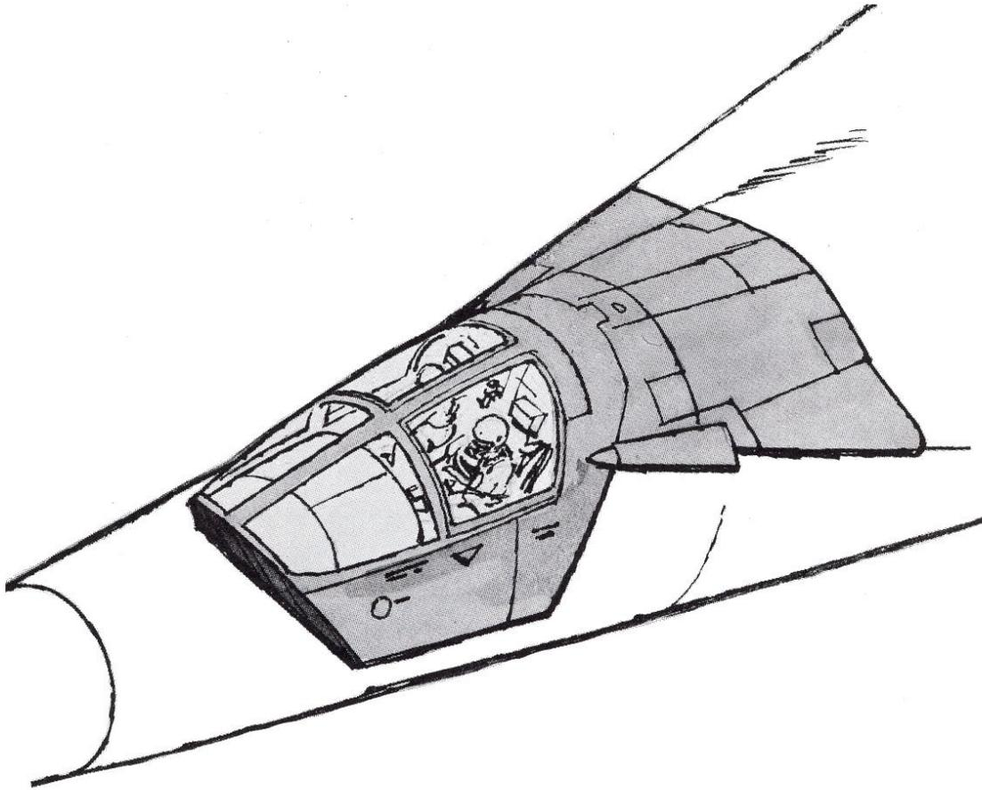
**Crew Module.** For crew comfort and safety, the F-111 is equipped with a special crew module that essentially is a self-contained vehicle within the aircraft. Developed by McDonnell Aircraft Corporation as a subcontractor to General Dynamics, the module serves as an operating compartment for the crew. If required, it also can serve as an escape system and as a survival shelter.
