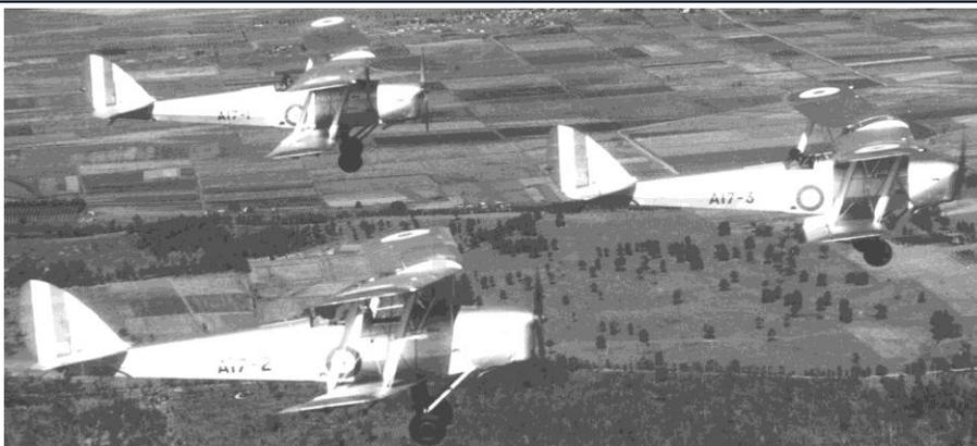
1939 – A17-1, A17-2 and A17-3, the first Tiger Moth production from DHA at Bankstown: overall *Aluminium K3/162*, iaw AGI C.11 in SEP 1939, with prewar 'Type-A' National Markings, but with rudder striping.
