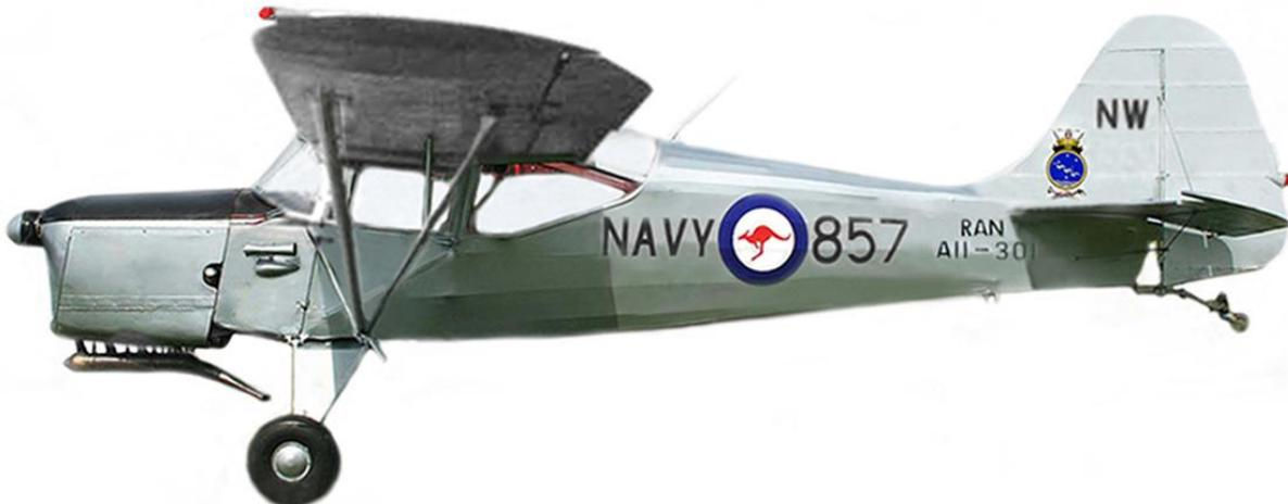
'Half-size' RAN serials: 1956 RANAMO gives tiny 'half-size' serial number fonts as 4" x 2.5" (0.6" stroke).<sup>77</sup> Nowra code numbers were more legible: code numbers 9" x 6" (1.25" stroke), "NAVY" 7" x 5" (1").
