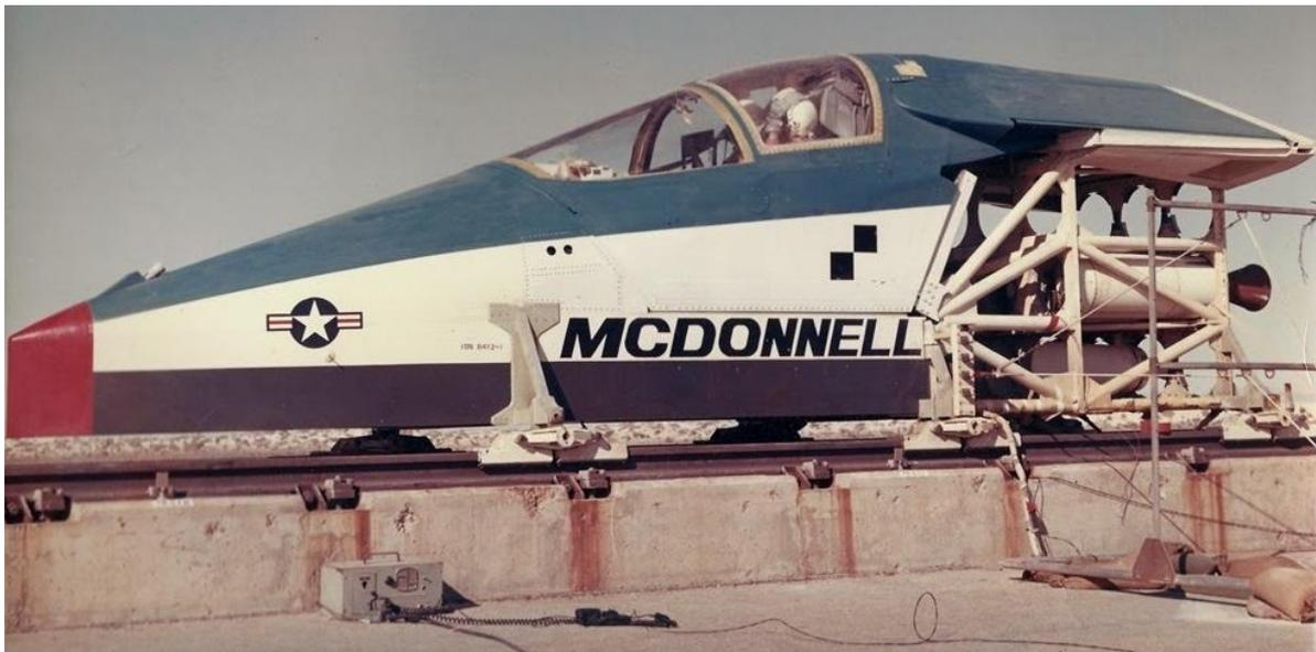
Initial sled testing with a dummy was carried out in the early sixties: Credit: McDonnell Aircraft Corporation<sup>102</sup>
