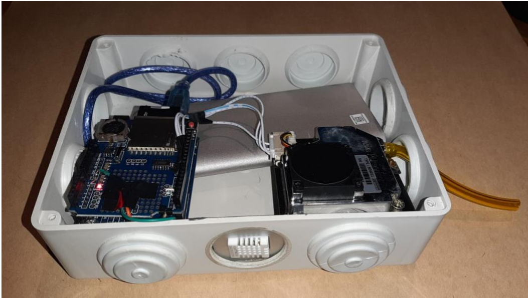
Figure B4. Prototype of the air quality sensors assembled for this study.
